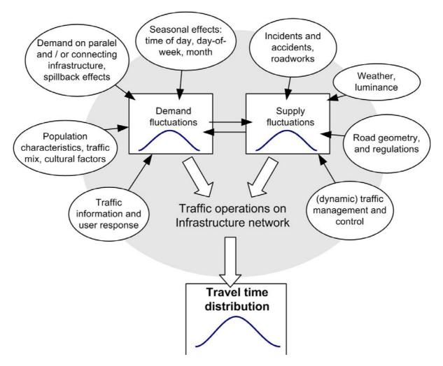
Figure 9: Schematic overview (not exhaustive) of factors influencing the distribution of travel times. Source: van Lindt et al (2008, Figure 1).
